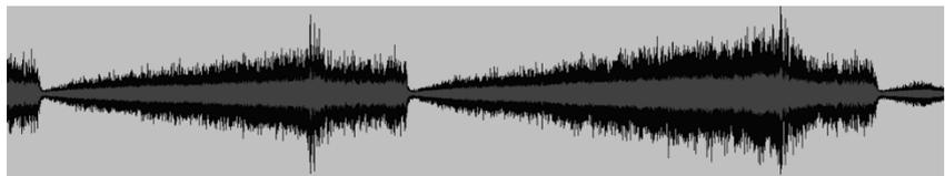
dependent on the load on the trap. Measurement of time intervals allows the monitor to estimate the current condensate load if design parameters are known.
