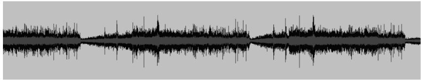
dependent on the load on the trap. Measurement of time intervals allows the monitor to estimate the current condensate load if design parameters are known. Time between discharges may vary widely between long intervals and short ones.
